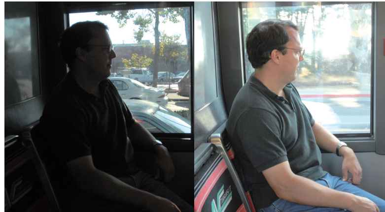
▲ Analog CCD cameras struggle to serve intelligent video applications due to their limited dynamic range.
